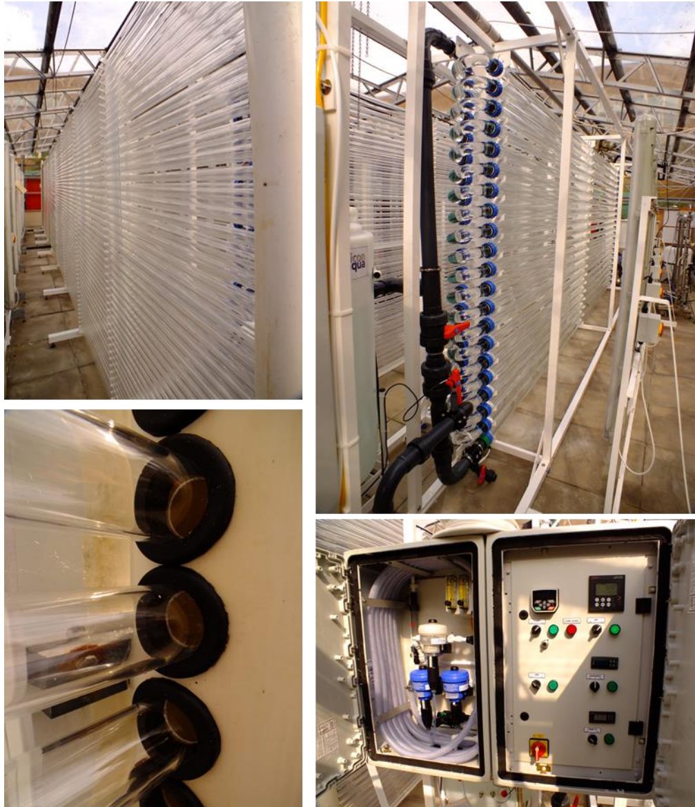
Fig. 4.6. Commercial horizontal tube bioreactors; Varicon Biofence (left) and Phyco-Flow (right). The Biofence comprises narrow bore acrylic tubes that are grouped together for liquid flow, while the Phyco-Flow comprises larger bore but glass tubes which are linked end-to-end by curved connectors for an improved flow. The cleaning brush for the Phyco-Flow (see Fig. 4.1, lower panels) is housed between the orange taps in the dark vertical tube. To the left of that, and extending out of sight, is the gas-exchange tank which is particularly important in horizontal bioreactor configurations. Lower right shows the control panel and the dosing system for sterilizing the system prior to inoculation.
