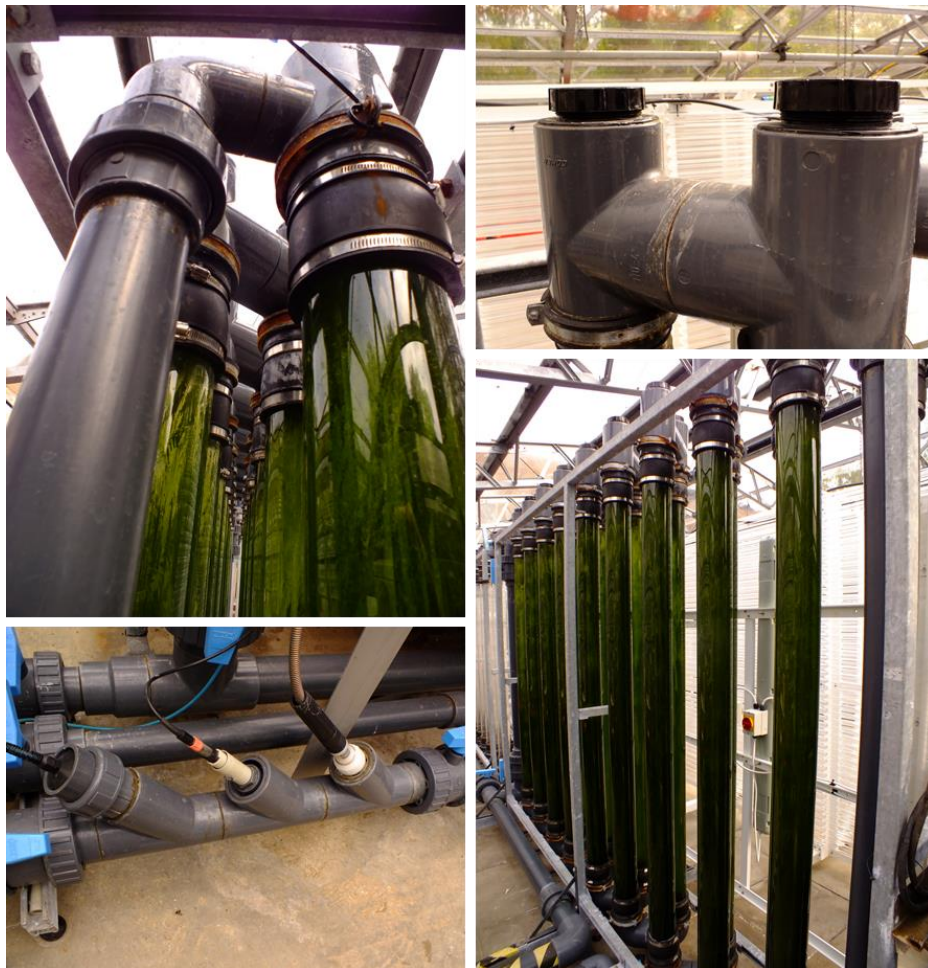
Fig. 4.5. Custom made multiple vertical-tube reactor with a total volume of 1000L. The diameter is 12cm. These acrylic tubes are connected at top and bottom so the culture is pumped through the whole system. Top-right shows the top caps, with degassing vents. Bottom-left shows the pH and \text{O}_2 sensors in the return-from-pump branch of the system. Although of potentially infinite expansion, this reactor design is not amenable to easy-cleaning, requiring the removal of the upper unions and the use of a brush (see upper panels of Fig. 4.1).
